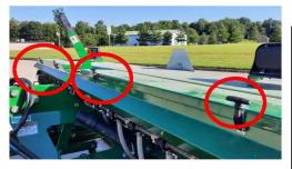
Are there two red brackets with pins? Is the electric connections intact? Is the top latch intact?
