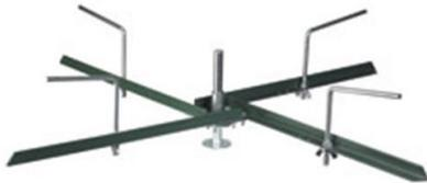
Used to install high-tensile wire fences. Load the wire and set on the ground. Walk away pulling the end of the wire and it will spin, preventing your wire from tangling. Slow down gradually before stopping to prevent over-spinning and tangling. Can also be used to rewind wire in the field.
