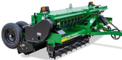
The NTS26 Series No-Till Seeder is equipped with a main and small seed box, making quick work of renovating pastures, reclaiming rights-of-way, and planting food plots. Metering is ground-driven by the rear packer-roller. The NTS's tillage aggressiveness is controlled by angling the front spiked rollers. Protected by a metal wind shield, seed is directed to the ground below and gently pressed into the soil with the rear cast packer.
